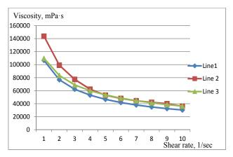
Fig. 1. Rheogram of the flow of gel samples of a dental product.
