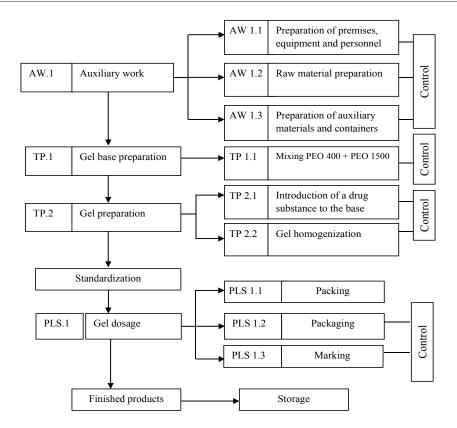
Scheme. Technological scheme for the production of dental gel «Matripin-Dent».
