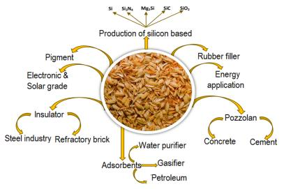
Fig. 2. Principal directions for the recycling of rice husk.
