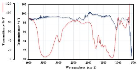
Fig. 6. FTIR spectra of RH (red) and SiO<sub>2</sub> (blue).
