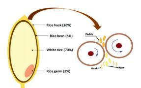
Fig. 1. Paddy rice grain (left) and its products after husking.
