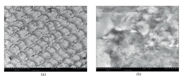
Fig. 4. SEM images of (a) rice husks before heat treatment (a) and (b)  $SiO_2$ .
