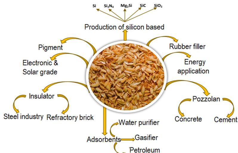
Fig. 2. Principal directions for the recycling of rice husk.
