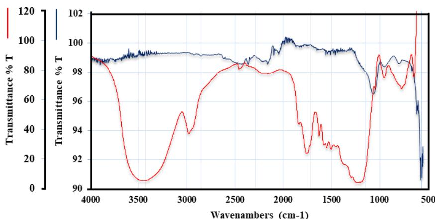
Fig. 6. FTIR spectra of RH (red) and SiO<sub>2</sub> (blue).
