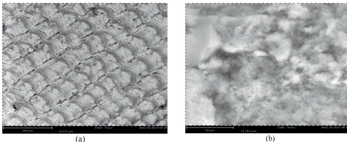
Fig. 4. SEM images of (a) rice husks before heat treatment (a) and (b) SiO<sub>2</sub>.
