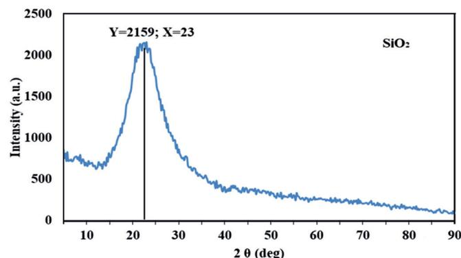
Fig. 3. X-ray diffraction pattern of silica.
