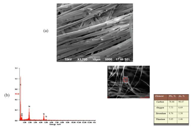
Fig. 6. SEM (a) and EDS (b) of aligned SrTiO<sub>3</sub>/PAN based fibers. This figure is reprinted from [57], with permission from Elsevier, 2019
