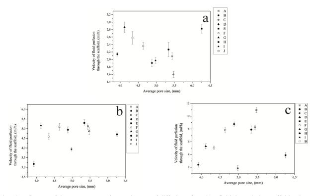
Fig. 13. Influence of the average pore size on the rate of diffusion of nutrient fluid through the scaffold at its rotation rate of 6 (a), 12 (b) and 24 (c) rpm.
