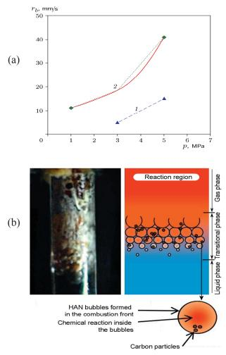
Fig. 2. a – Calculation of linear combustion rate of studied compositions depending on initial pressure system: 1 – HAN/CMC, 2 – HAN/CMC + activated carbon; b – combustion wave propagation at burning of HAN in liquid phase at  $p_0 = 6$  MPa.
