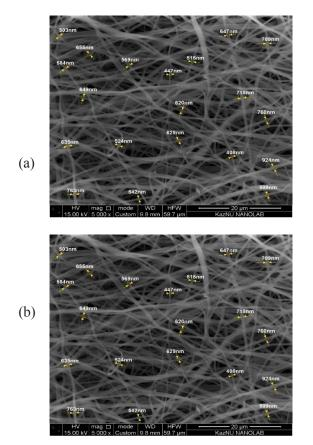
Fig. 11. SEM images of samples of carbon fibers based on coal tar pitches and PAN (a) after stabilization and (b) after carbonization.
