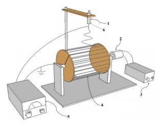
Fig. 10. General diagram of the electrospinning installation: 1 - syringe; 2 - motor; 3 - motor speed controller; 4 - drum collector; 5 - high-voltage power supply; <math>6 - needle.
