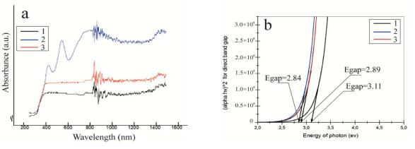
Fig. 7. Absorption and reflection spectra (a) and values of the bandgap (b) of synthesized composite photocatalysts:  $SrTiO_3/PAN/Fe_2O_3 - 1$  (black line);  $SrTiO_3/PAN/CuO - 2$  (blue line); and  $SrTiO_3/PAN/Cr_2O_3 - 3$  (red line). This figure is reprinted from [59], with permission from MDPI, 2020.
