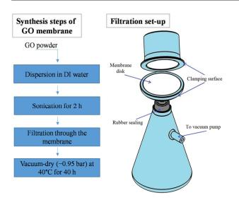
Fig. 3. The scheme of synthesis steps of GO membrane and filtration set-up.
