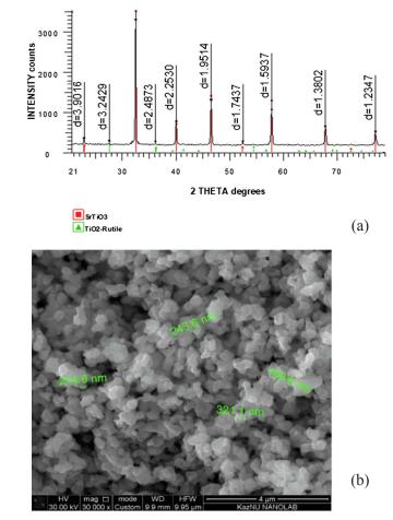
Fig. 5. X-ray pattern (a) and SEM (b) of the synthesized  $SrTiO_3$  powder. This figure is reprinted from [57], with permission from Elsevier, 2019.
