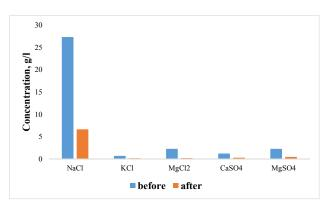
Fig. 4. Concentration of salts before and after filtration.
