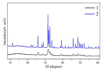
Fig. 12. X-ray diffraction patterns of HAP: 1 - HAP particles without post-thermal treatment; 2 - HAP particles with post-thermal treatment at a temperature of 1100 ° C for 3 h.
