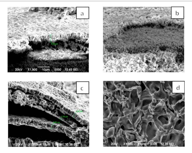
Fig. 8. SEM images of porous CoTiO<sub>3</sub> calcined at: a - 600 °C, b - 650 °C; c - 700 °C; d - 800 °C. This figure is reprinted from [60], with permission from Elsevier, 2021.
