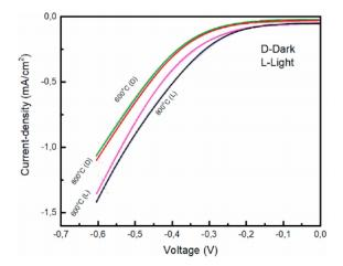
Fig. 9. I–V curves of porous  $CoTiO_3$  in 0.5 M KOH solution.
